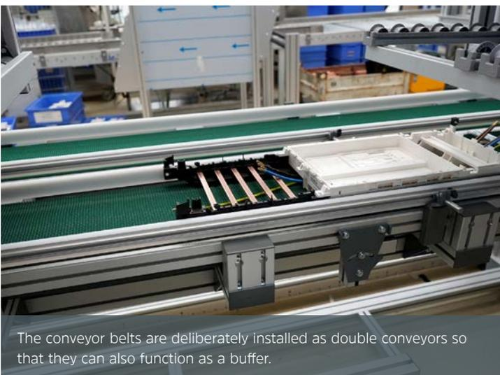
The conveyor belts are deliberately installed as double conveyors so that they can also function as a buffer.
