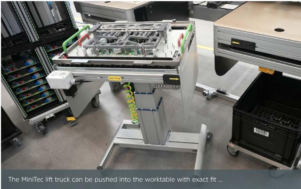
The MiniTec lift truck can be pushed into the worktable with exact fit ...
