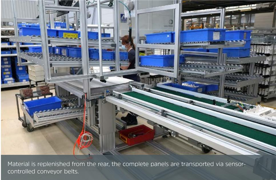
Material is replenished from the rear, the complete panels are transported via sensor-controlled conveyor belts.
