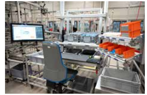
An ergonomic assembly workstation and the interactive assistance system form a functioning unit at Martor.
