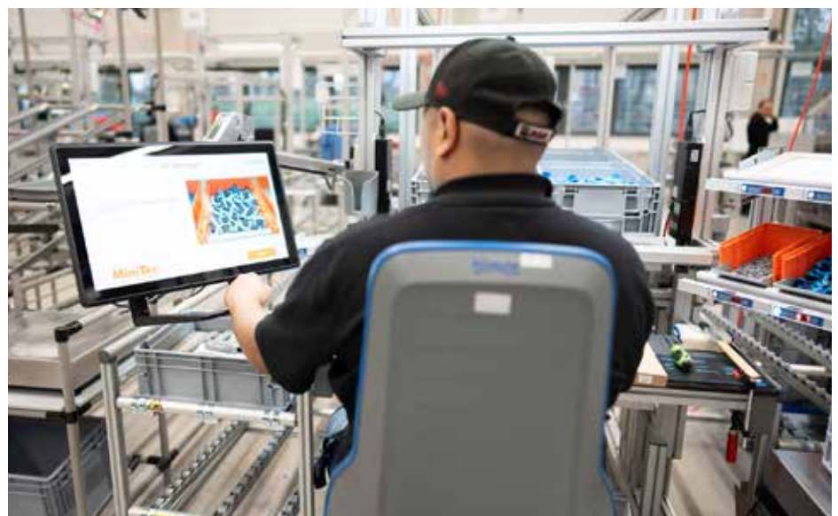
The worker is guided through the assembly process step-by-step via the touchscreen.
