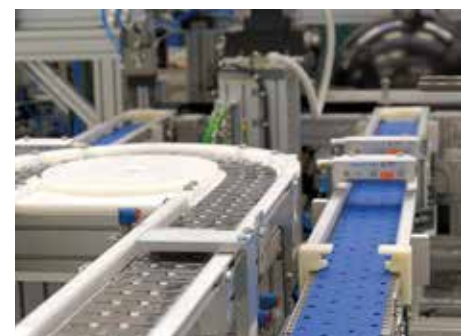
Conveyors with linked link chains are ideally suited to curved sections, rises or complex layouts.
