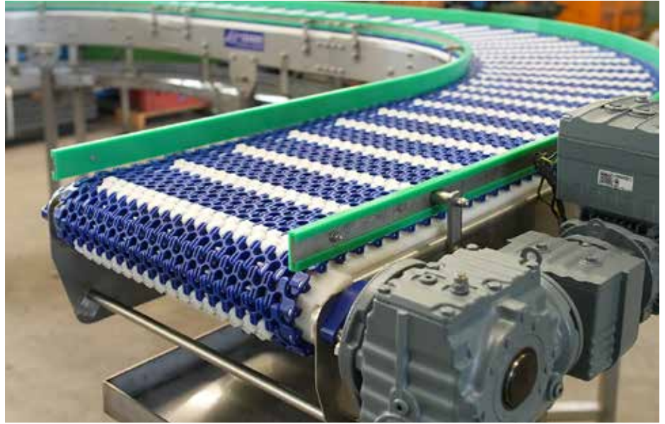
Modular belts can also master curves, rises and changes in level.
