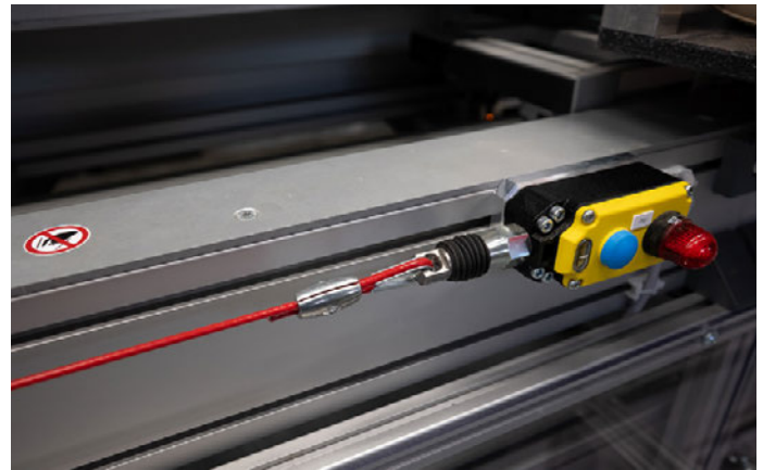
The emergency cable pull is easy to reach in case of malfunctions.
