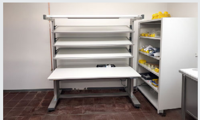
Height-adjustable ESD table with adjustable shelves and integrated lighting.
