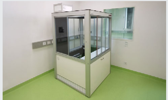
Device enclosure for mass spectrometer with controlled exhaust air and sound insulation.
