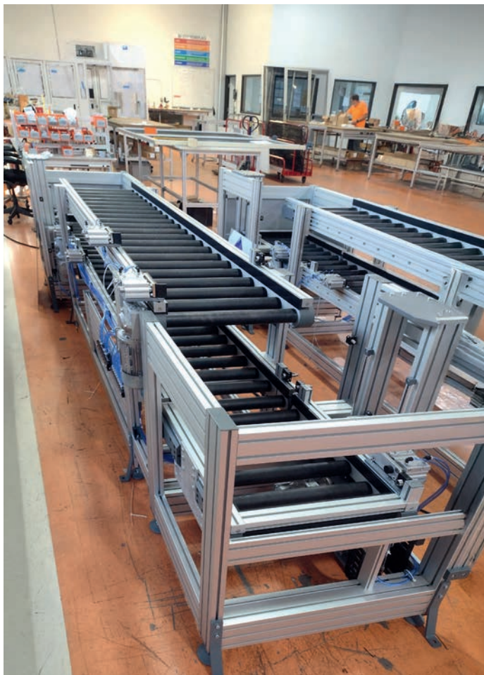
Conveyor section for the transport of valve trims.
