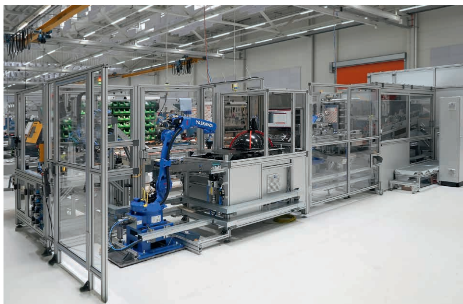
Robots can move workpieces to stationary quality test sensors.
