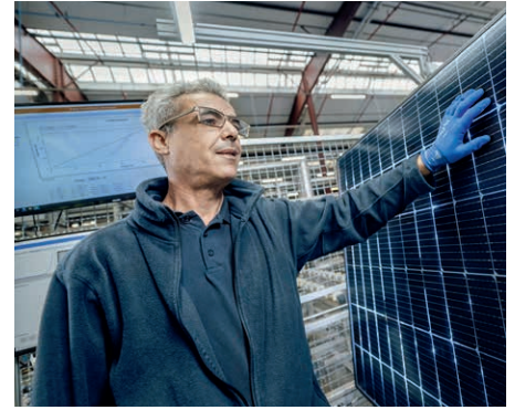
Visual inspection: The employee compares the information on the control screen with the panel.
