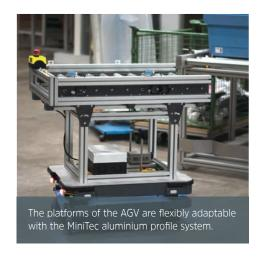
The AMRs therefore integrate themselves into the processes as a type of flexible conveying technology and form a link between the existing conveying systems. Possible adaptations to changing circumstances can be implemented easily at any time. The installed sensors even enable the robot to independently open doors that it has to overcome on its way to its destination point. That makes use of the AMR even more useful for us.
