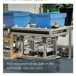
The integration of the robot in the warehouse was very simple, as it had already long since been semi-automated with conveyor technology. The existing conveyor technology therefore only had to be supplemented with a transfer point, at which the AGV can hand over the SLCs.
