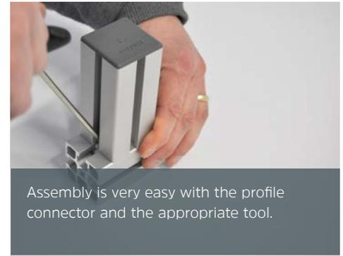
Assembly is very easy with the profile connector and the appropriate tool.
