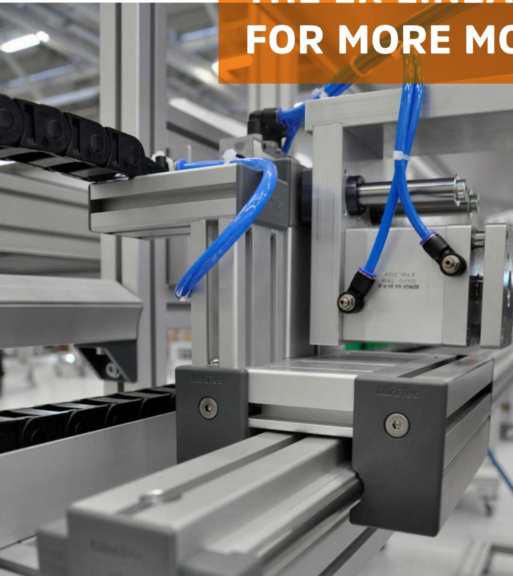
MiniTec modular profile system. This ensures that the respective linear unit fits seamlessly into the construction.
