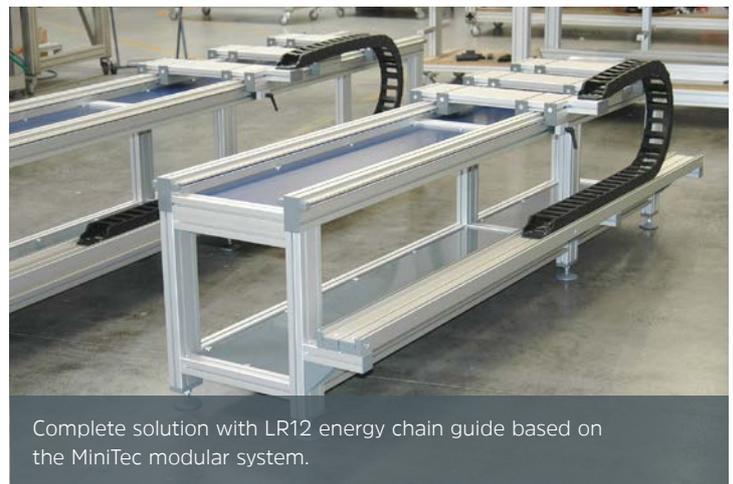
Complete solution with LR12 energy chain guide based on the MiniTec modular system.
