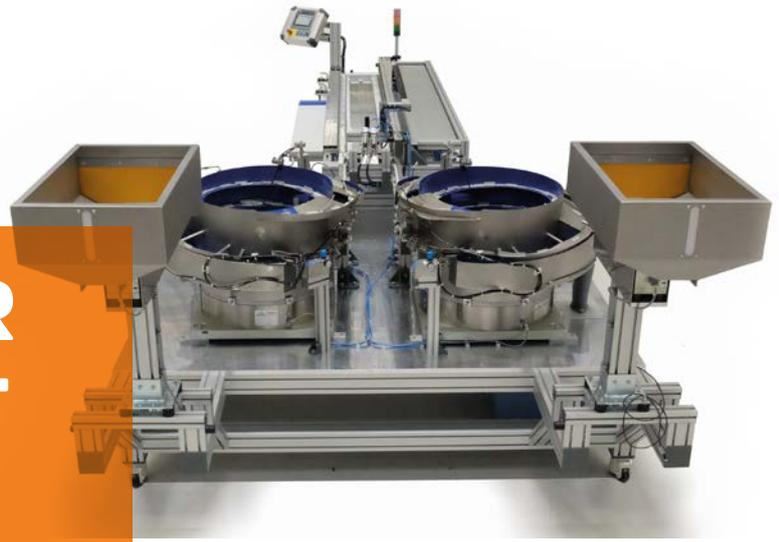
**Efficiency and speed are also required in switch cabinet construction. Friedrich Lütze GmbH, which specialises in electronic and electrotechnical components, have opted for an automation solution from MiniTec. The new system fits components into aluminium strips for cable routing. It enables higher production volumes and a significantly more efficient assembly of switch cabinets.**
