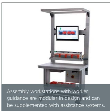
Assembly workstations with worker guidance are modular in design and can be supplemented with assistance systems.
