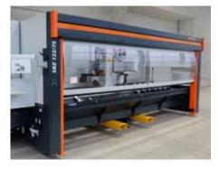
The new 5-axis machining centre enables complex profile machining.
