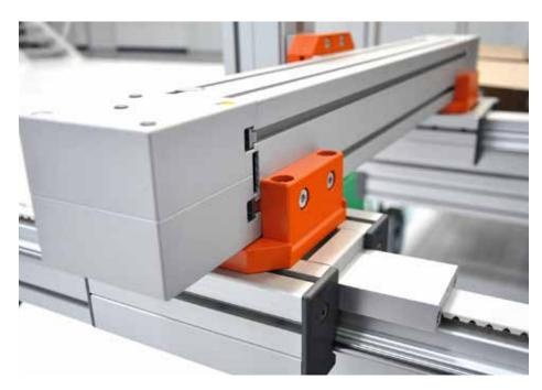
With the help of adapters, all linear axes can be easily and economically combined to form multi-axis systems.
