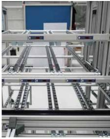
Pick to light strips indicate to the worker, which material they need for the pending assembly process
