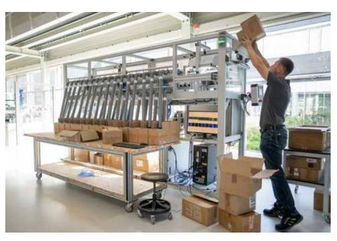
The system during the test run – a Meprovision employee fills it with golf balls. An automatic step conveyor will be used here later.
