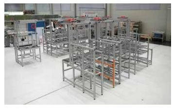
The U-shape of the system allows fluid, assembly in the team based on division of labour (task segmentation).
