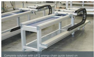
Complete solution with LR12 energy chain guide based on the MiniTec modular system.
